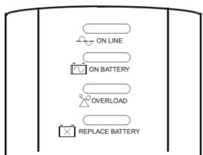
**On Line (green)** - is lit whenever AC power is powering the Battery Backup outlets.
