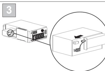
Slide the new battery into the battery compartment. Connect the battery wires to the terminals as follows:
