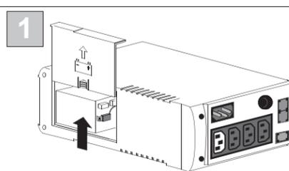
Place the unit on its side. Slide the battery compartment cover upward and off of the UPS.
