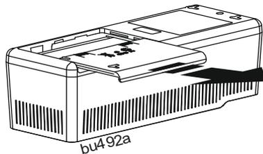
❸ Connect the battery cable securely to the battery terminal.
